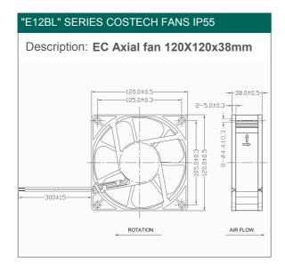
Casing material:Thermoplastic in black color, UL 94 V-0Impeller materialThermoplastic in black color, UL 94 V-0Protection degree:IP55, according to EN 60529 standard
